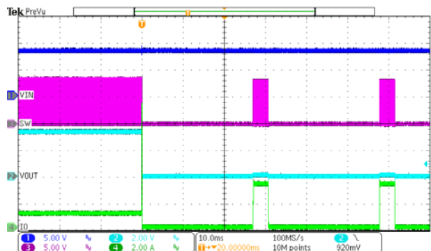
Figure 16. Over Current Protection (1A to hard short)
