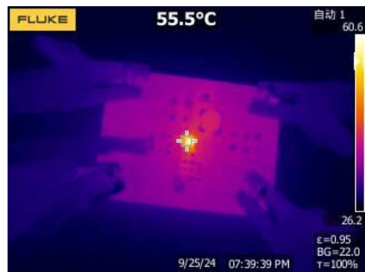
Figure 20. Thermal, V_{IN}=5V, V_{OUT}=1.2V, I_o=2A
