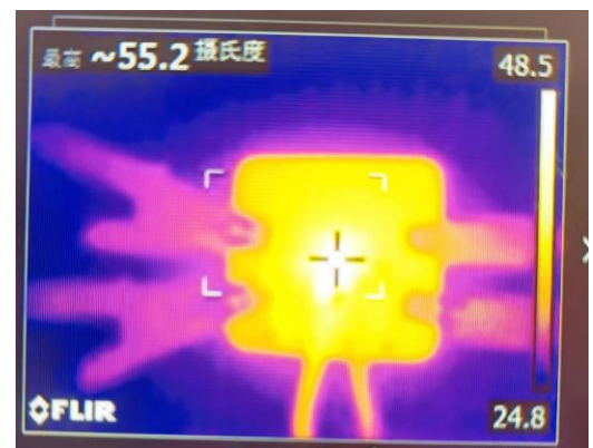
Figure 20. Thermal, 12VIN, 3.3Vout, 3A(SOT563)
